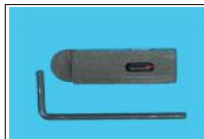
Figure 8: The Adjustable Secondary Standard includes a fluorescent rod that provides an extremely stable signal.
