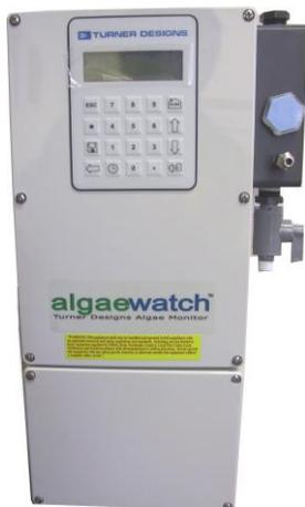
**AlgaeWatch** is a fluorescence sensor designed to monitor the level of chlorophyll containing cells in fresh water. The **AlgaeWatch** continually senses the concentration of chlorophyll *a*, an indication of algal biomass, in the sample water.
