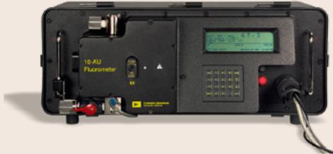
Further development resulted in an improved method called QFT2. QFT2 involves a two-point fluorescence measurement that yields estimates of both absolute oil quantity (weight % oil) and oil type (API gravity). The speed, accuracy and ease of application make QFT2 a practical tool for the determination of oil concentration and API gravity at the well-site.
