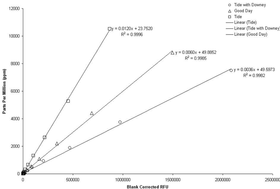
**Figure 1 (left):** Optical Brightener Module's fluorescence responses (RFU's) of varying concentrations from three different detergents. A linear regression for each detergent is shown with its respective slope equation and r-squared value.
