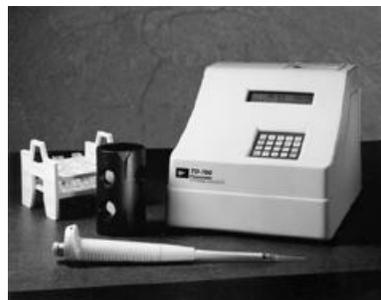
The TD-700 Laboratory Fluorometer
