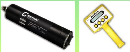
Turner Designs C-sense submersible pCO<sub>2</sub> and DataBank Datalogger
