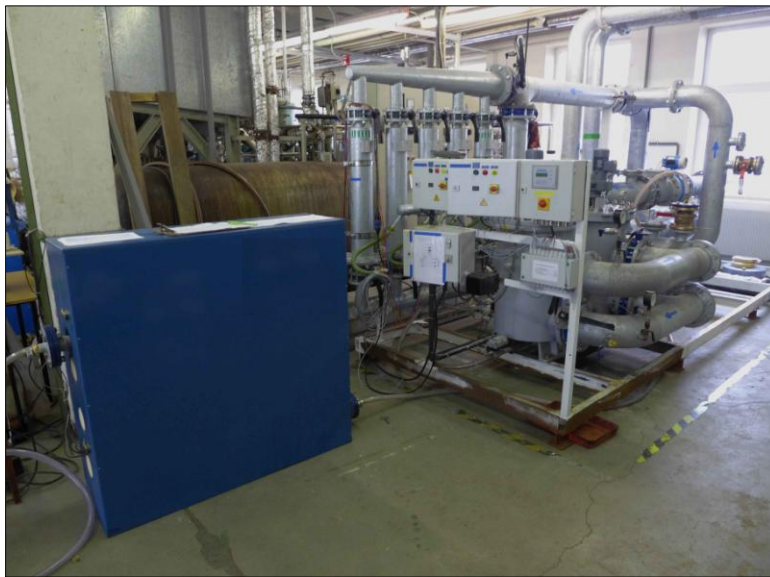
Ultrasound treatment system (blue box) tested at the Institute for Nautics and Maritime Technologies, Flensburg University of Applied Sciences, Germany
